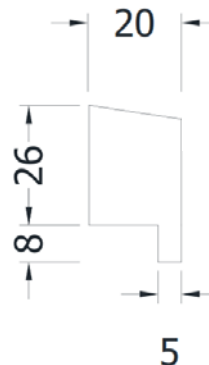
Bead dimensions for 54mm thick leaf
